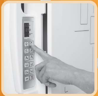
Bucky with fixed detector has all control buttons such as display, incl. SID, altitude and RED display
